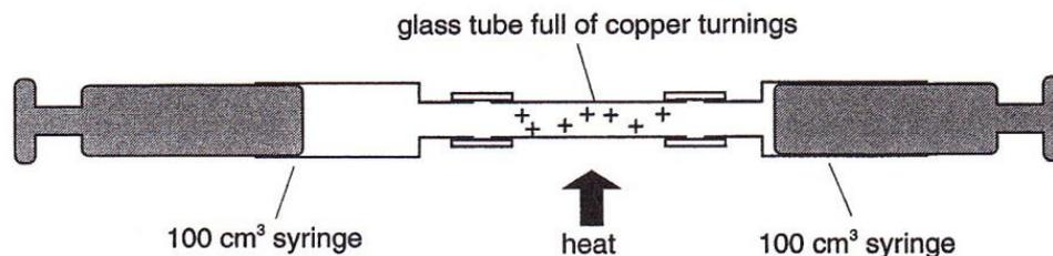
The gas was passed backward and forward over heated copper turnings. The results obtained were used to plot the graph.
