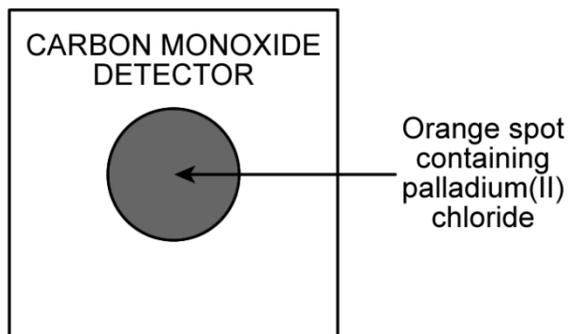
The orange spot turns black if there is a high concentration of carbon monoxide in the air.
