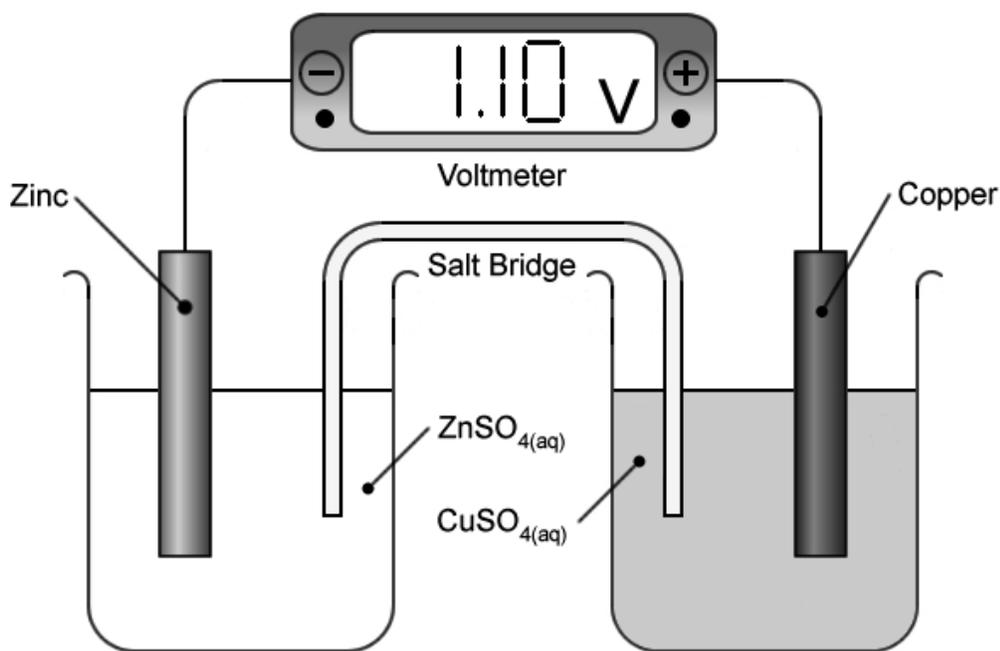
**Figure 2.** A simple electrochemical cell or battery.
