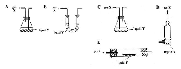
5. Substance X melts at 53°C and boils at 100°C. It does not dissolve in water and it does not react with water. Which diagram shows the method most suitable for separating X from a mixture of X and water?
